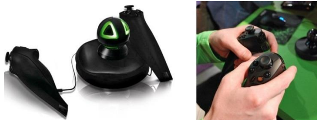
Figure 2: The six degree-of-freedom Razer Hydra interface. (Courtesy of Sixense TrueMotion)
