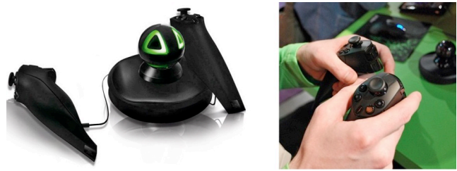
Figure 3: The bimanual Razer Hydra interface
